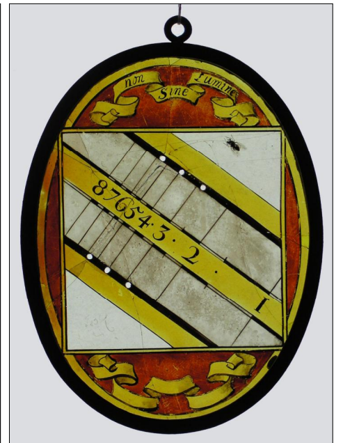
Fig. 6. The Non Sine Lumine dial, a direct west dial designed like a mathematical scale; the style of the inscription appears on a number of dials attributed to John Oliver. (Private collection).
